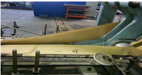
Fig. 7. First steps in sacks forming (overlapping)
