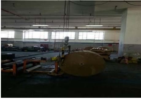
Fig. 3. Set the craft paper roller in the beginning of the production line
